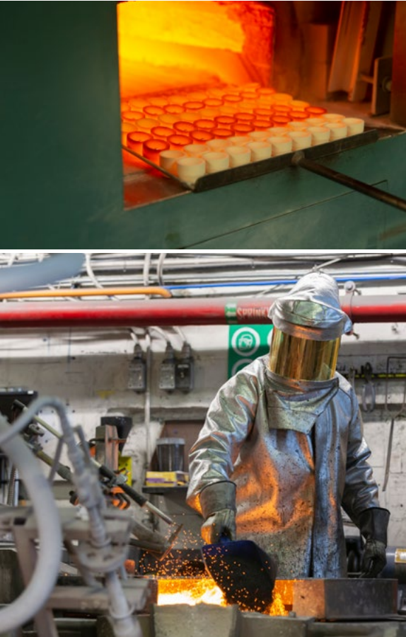
Top: Refined gold samples undergoing fire assay. Bottom: A refinery operator pouring pure silver bars at the Mint's Ottawa facility.
